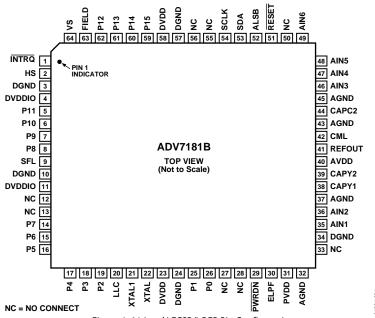
Figure 4. 64-Lead LFCSP/LQFP Pin Configuration
