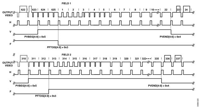
Figure 25. PAL Default (BT.656). The Polarity of H, V, and F is Embedded in the Data
