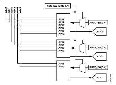
Figure 5. Internal Pin Connections
