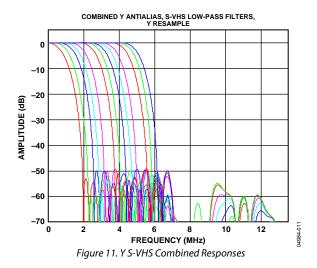
The filter plots in Figure 11 show the S-VHS 1 (narrowest) to S-VHS 18 (widest) shaping filter settings. Figure 13 shows the PAL notch filter responses. The NTSC-compatible notches are shown in Figure 14.
