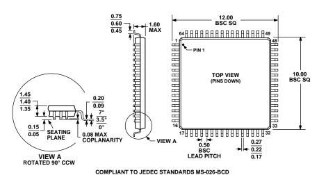
Figure 47. 64-Lead Low Profile Quad Flat Package [LQFP]
