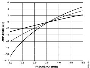
Figure 35. NTSC IF Compensation Filter Responses
