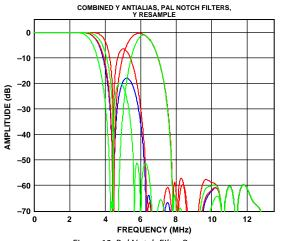
Figure 13. Pal Notch Filter Response
