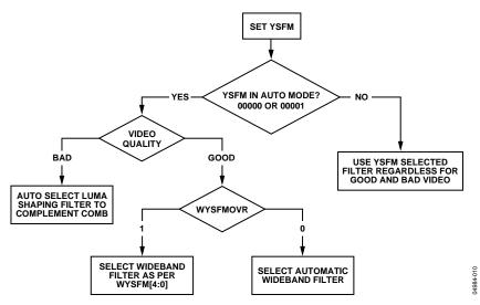
Figure 10. YSFM and WYSFM Control Flowchart
