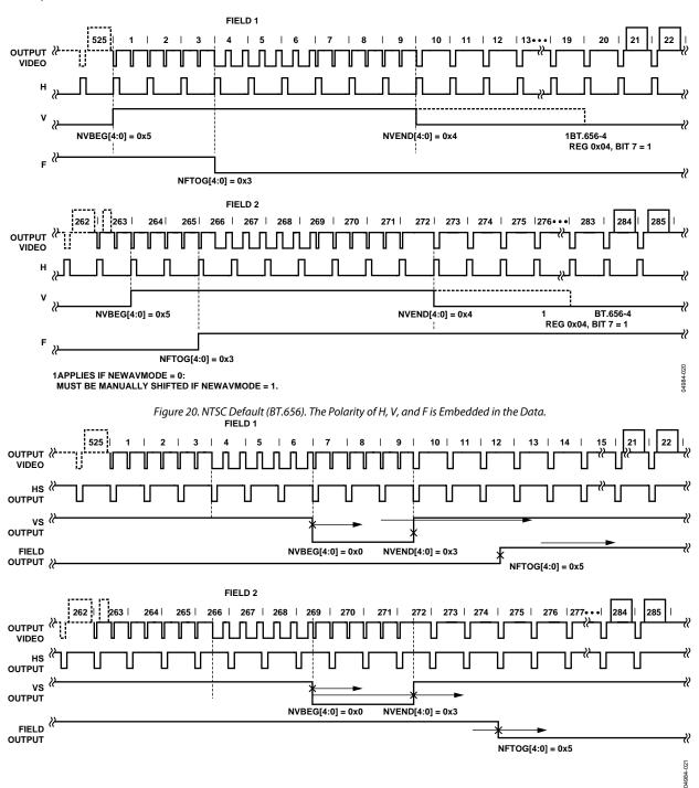
Figure 21. NTSC Typical VSync/Field Positions Using Register Writes in Table 54.
