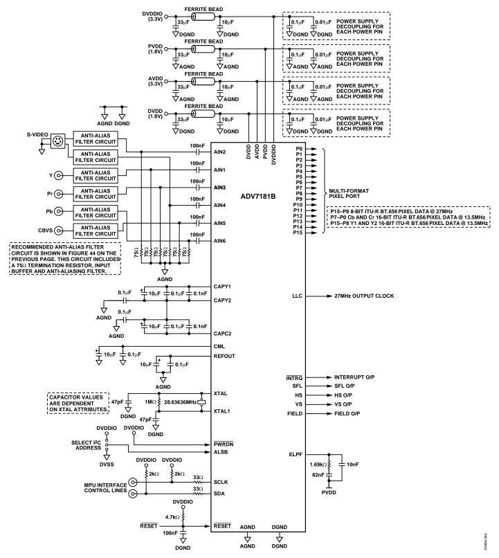
Figure 45. Typical Connection Diagram
