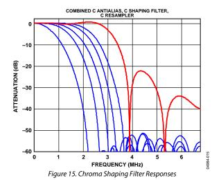
Figure 15 shows the responses of SH1 (narrowest) to SH5 (widest) in addition to the wideband mode (in red).
