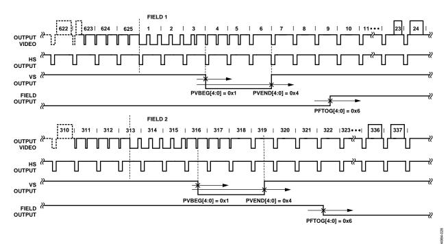
Figure 26. PAL Typical VSync/Field Positions Using Register Writes in Table 55
