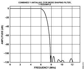
Figure 12. Y S-VHS 18 Extra Wideband Filter (CCIR 601 Compliant)
